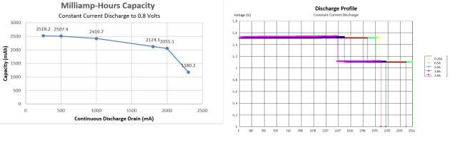
Discharge Capacity (mAh)
