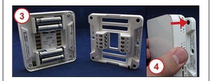
5. When the batteries are inserted correctly, the display screen will become active.
