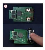
6. When the battery is inserted correctly, the red light on the circuit board will illuminate.
