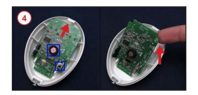
Insert one CR123A battery by aligning the positive (+) and negative (-) ends of the battery with the positive (+) and negative (-) indicators on the circuit board, then pressing the battery into the battery clasps.
