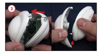
Remove the green circuit board by pushing forward on the catch and gently lifting the circuit board out of the Sensor body. The battery compartment is located on the back of the circuit board.
