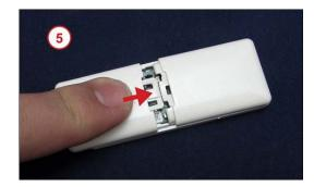
6. When the battery is inserted correctly and the cover is reattached, the red light on the front of the Sensor will light up.
