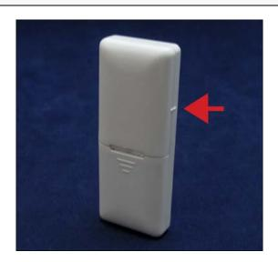
1. Locate the small horizontal raised lines in the shape of a pyramid on the Sensor.
