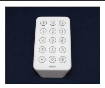
Grasp the sides of the keypad and slide it upwards until it releases from the back cover.
