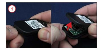
Gently remove the circuit board and insert one CR2032 battery into the battery slot matching the direction of the positive (+) placement indicator. If you don't see an indicator, insert the battery with the positive (+) side facing away from the circuit board.
