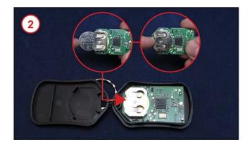
Align the circuit board with the Remote keypad as shown below and gently place the circuit board with the inserted battery back into the Remote. The battery faces the back of the Remote.
