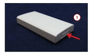
2. Move your fingertip down while holding the front of the Sensor to pry the cover away from the Sensor body.
