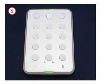
Confirm that the low battery alert has resolved. You should also ensure that keypad events such as arming or disarming registers as an activity on your system.
