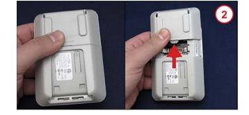
**Take a Look.** If a battery is already present, remove it by using your fingertip to gently pull one end of the battery up until the battery is loose and you can pull it free from the slot.
