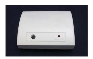
1. Hold the Glass Break Sensor with both hands and use your thumb to pull the cover away from the Sensor body.
