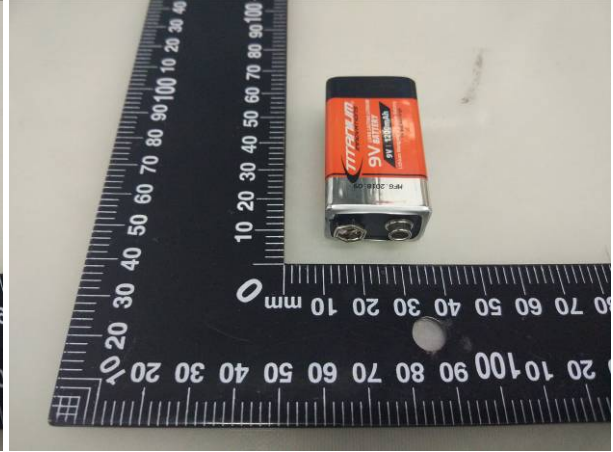
Battery/电池 (CR9V 9,0V 1200mAh)
