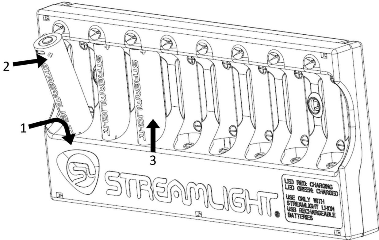
1. Insert the negative end of the battery pack into the spring end of the charger cavity (polarity is marked in each battery cavity).
