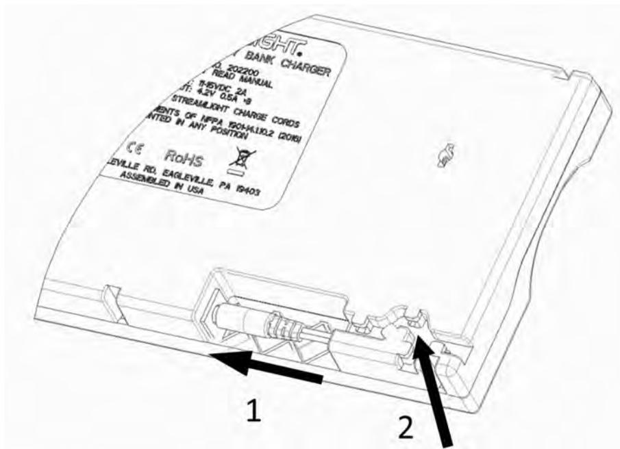
1. Insert the 2.5mm barrel connector from the cord into the power jack on the back of the charger.
