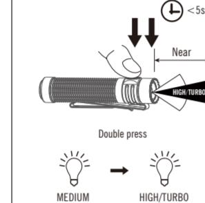
(Note: After the obstruction caused downshift stage, the output brightness will remain Medium even after the obstruction is removed.)
