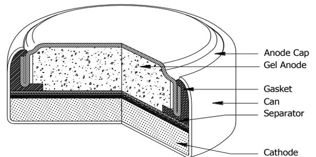
DESIGNED FOR USE ON CONTINUOUS LOW DRAIN
