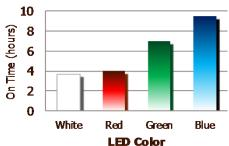
Flashlight mode tested according to ANSI/NEMA FL 1 Standards. Glow stick and flashing modes are area lights and not covered by the standard.
