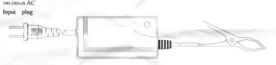
Output polarity: red clip is '+' and black clip is '-', Please make sure the battery you charged have a proper '+' and '-' connector.
